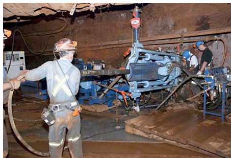
Figure 1: Diamond-drill core samples, taken 4850 feet underground in the former Homestake gold mine, will tell geologists and engineers where best to excavate drifts and caverns for the Sanford Underground Laboratory. (Bill Harlan/SDSTA)
