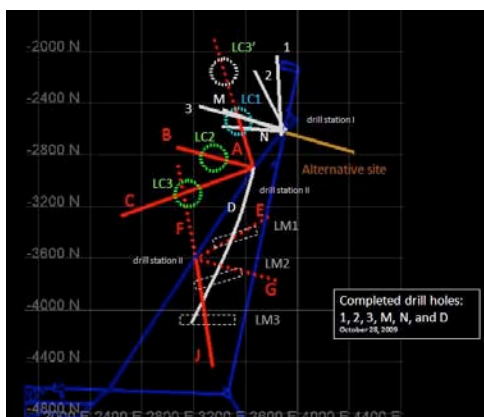
Figure 6: The planned geotechnical-coring plan on the 4850L is presented. Holes 1, 2, 3, M, N and D have been completed and logged. Hole C has extended beyond the LC3 location.
